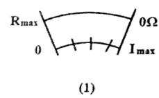
In figure (1) if resistance of device  $70\Omega$  and we connect to it a resistance R that cause pointer deflect to  $\frac{1}{2}$  its scale
